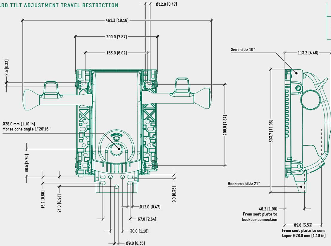
RECOMMENDED FIXING HOLES FOR BACK SUPPORT CONNECTION (WIDTH 90,0 mm [3,54 in])
