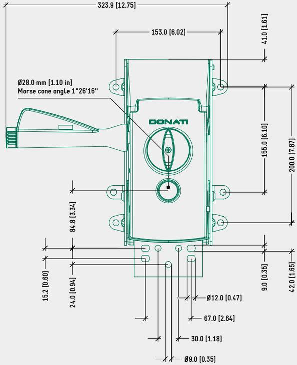
RECOMMENDED FIXING HOLES FOR BACK BAR CONNECTION (WIDTH 90,0 mm [3,54 in])
