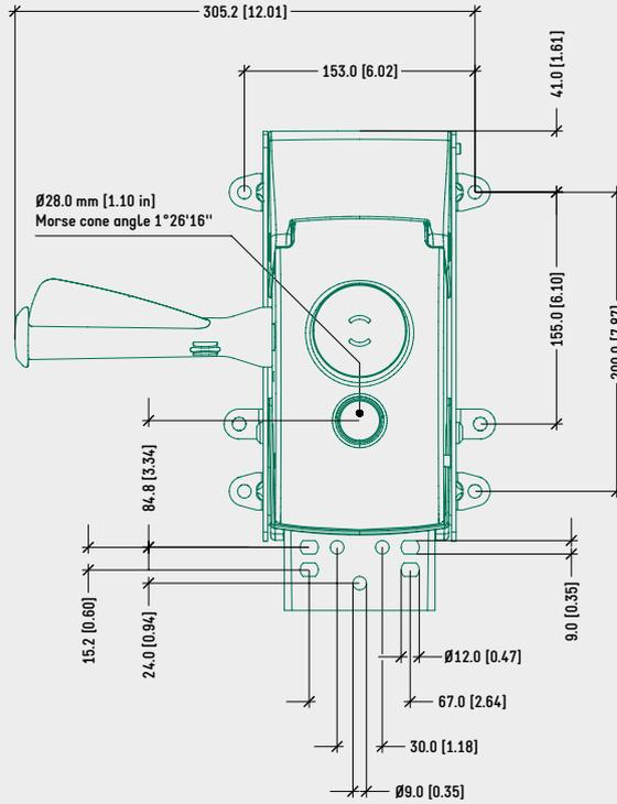
RECOMMENDED FIXING HOLES FOR BACK BAR CONNECTION (WIDTH 90,0 mm [3,54 in])
